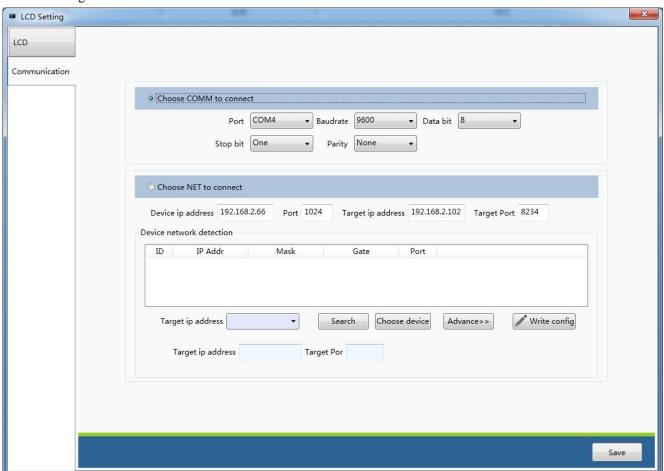
Open the communication setting, user can choose connect by COM or NET.If connect by COM, user only needs to set up COM port, Baud rate, Data bit, Stop bit and Parity. The COM port will be matched user's PC automatically, so choose COM1 if the port is COM1, Baud rate is 9600. Other options keep the same. Save the setting.
