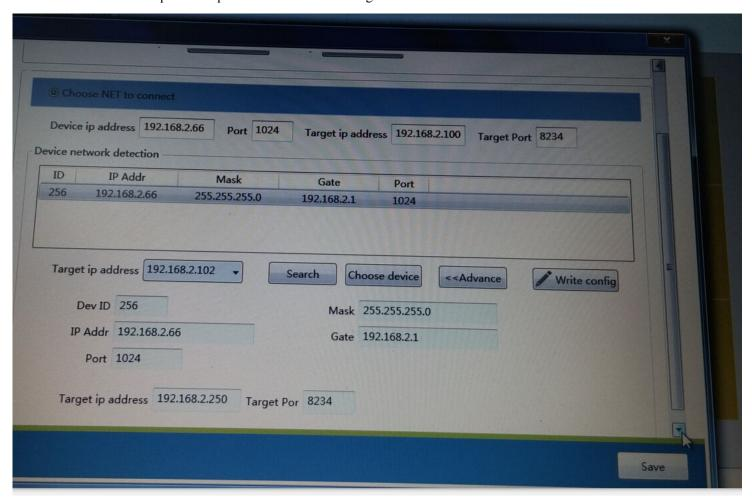
If connect by NET. Choose the PC IP address in Target IP address. Click Search button on right, then user can see the current on line video wall IP information in the Device network detection. Click Advance, and double click the video wall IP which need to be connected. Then user can revise and set up the IP information below. After finishing revision, click Write config then change the video wall management IP information .Click Choose device and Save.
