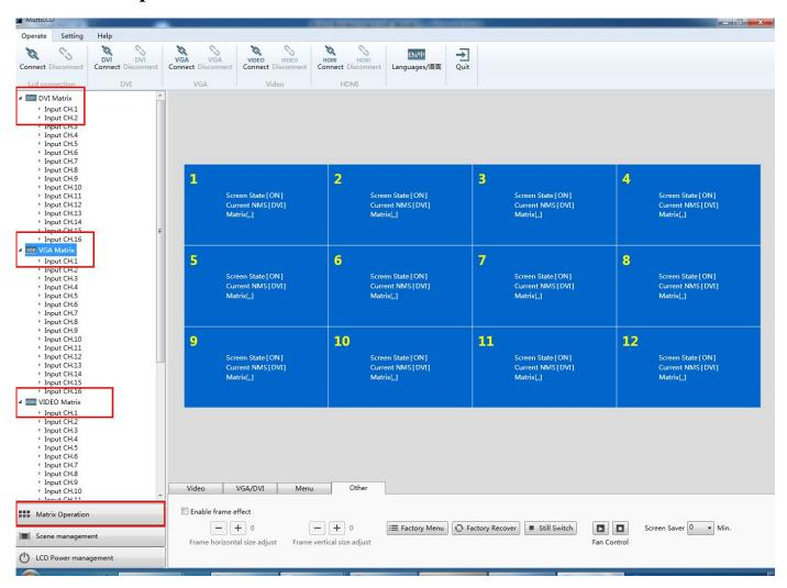
Set up the Configuration serial port and protocol of matrix in Setting. Click Matrix Operation button on left and list the input channel of the matrix. Choose the screens and double click the input channel, then the chosen screens will be transferred to the relative matrix input signal.
