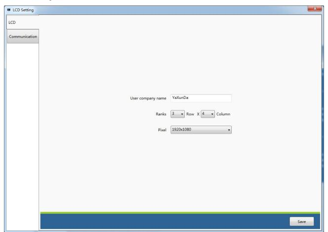
User can set up the LCD wall quantity and user name in this page. Set up the Row and Column quantity as per the current project requirement. Above Row 3 x Column 4. The LCD wall setting will be as below.
