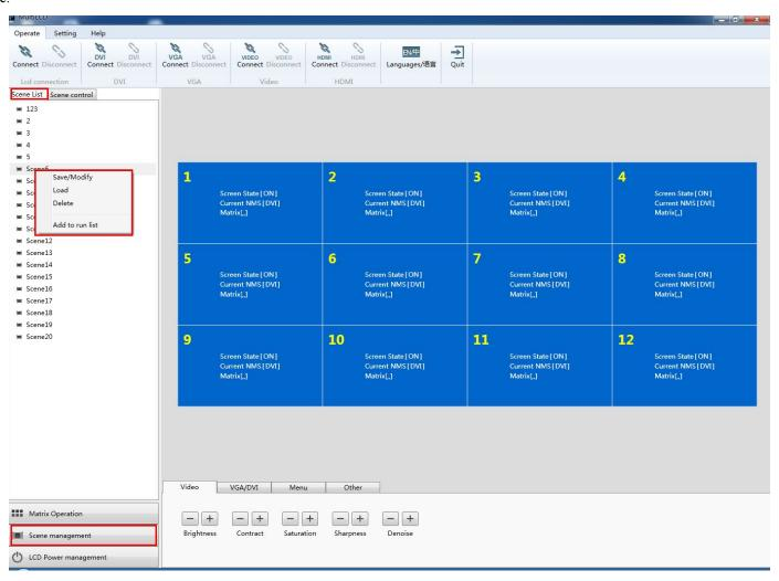
Click Save to save the current display state. Click load to load the saved scene. Click delete to delete the saved scene. Click add to list to add the saved scene to the list. Click Scene control on right to switch display the saved scene list. Choose the relative scene in list and click move up/ down to change the scene sequence.
